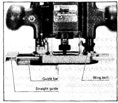
When cutting, move the tool with the straight guide flush with the side of the workpiece.
